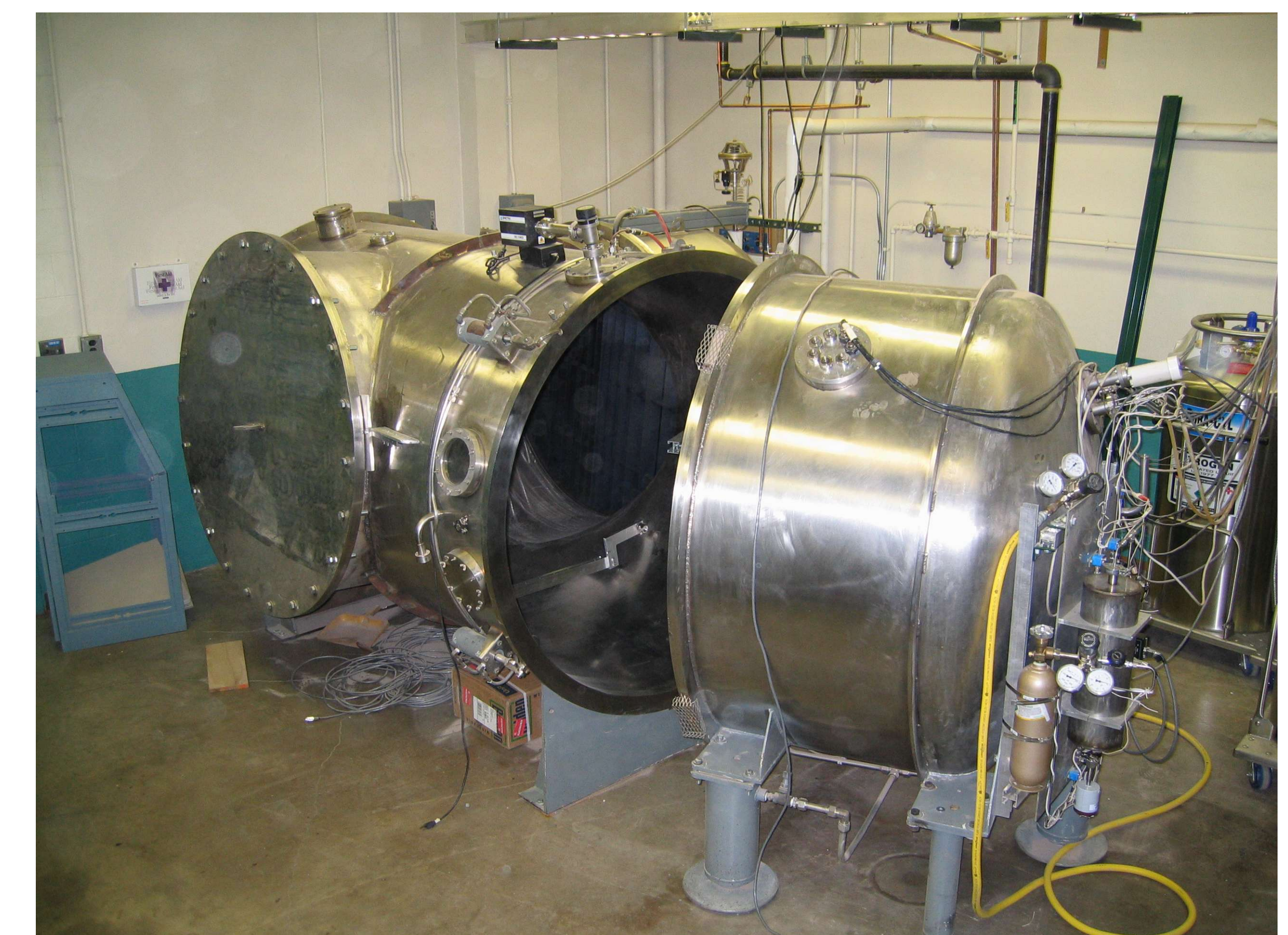
Space simulation chamber at the Ion Space Propulsion Laboratory
