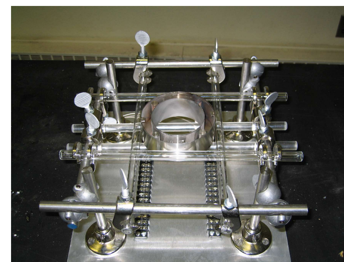
Mock-up anode being prepared for thermal testing.
